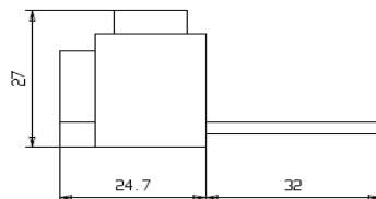
Feed-in terminal 50mm², Fork
